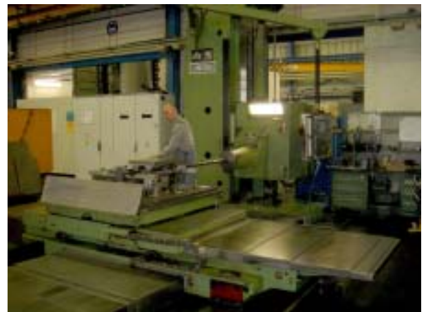
3177 UNION BFT 130/7 with CNC TNC 426 CB generally overhauled in 2000
