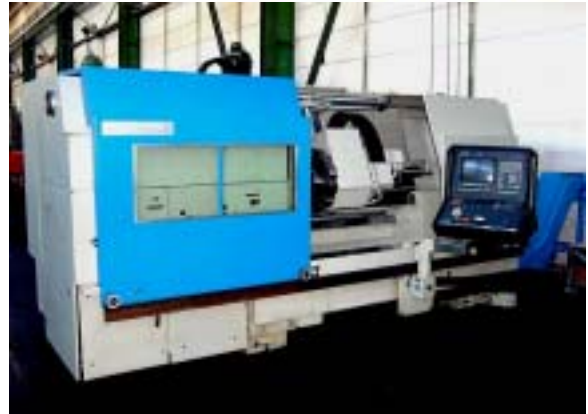
2947 WMW DFS 2/3 with CNC SIEMENS 820 with driven tools
